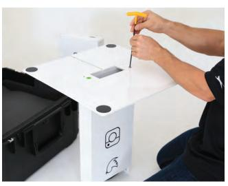
To properly orient the baseplate align the green dots on tube bottom and baseplate top.
