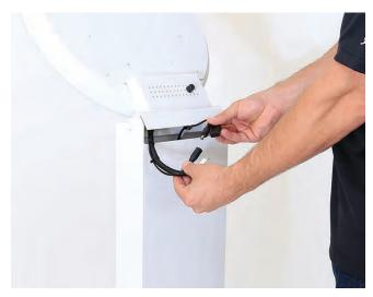
Push the head assembly forward to maximum forward angle to access the head pigtail and pivoter pigtail.
