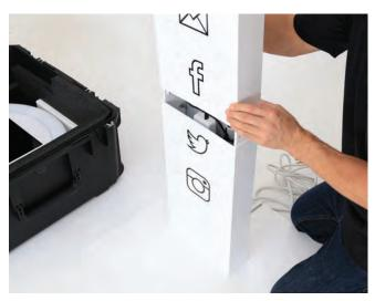
Place the top tube onto the bottom tube aligning green dots. Verify all cords are inside and not pinched.
