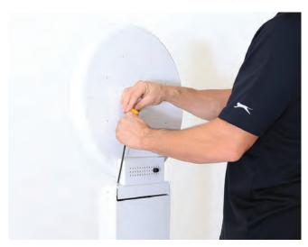
Install and tighten two bolts at the rear of the head assembly base to secure it to the pivoter.
