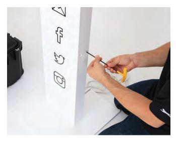
Install and tighten four bolts to secure top tube to bottom tube.
